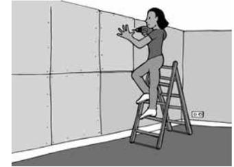
d) Walls that are painted or coated with primer must be completely dry and be sanded down (using 80-grit sandpaper) prior to assembly.
