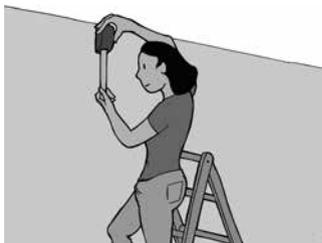
II. Use a long spirit level (and a straightedge if needed) and draw a horizontal line, for reference, across the entire width of the wall.
